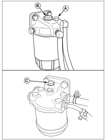
Figure 2. **Fuel System Priming**
